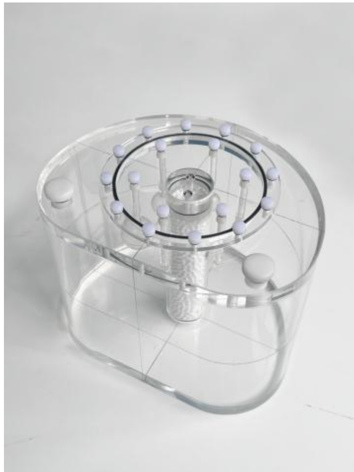
Figure A. 2 IEC body model (elliptical) schematic diagram
