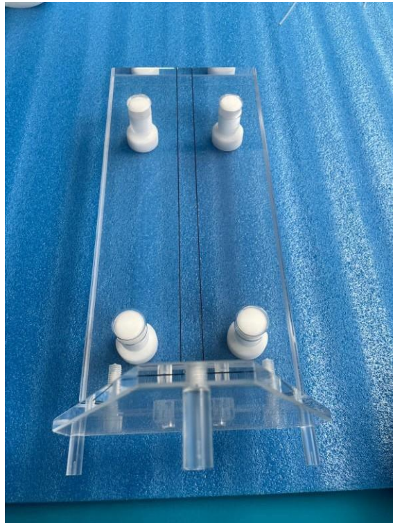
Figure A.4 Schematic diagram of the point source holder for spatial resolution monitoring
