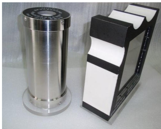
Figure 1: In-vivo temperature measurement body model KS205TW-2 and out-vivo temperature measurement body model KS205TW-1
