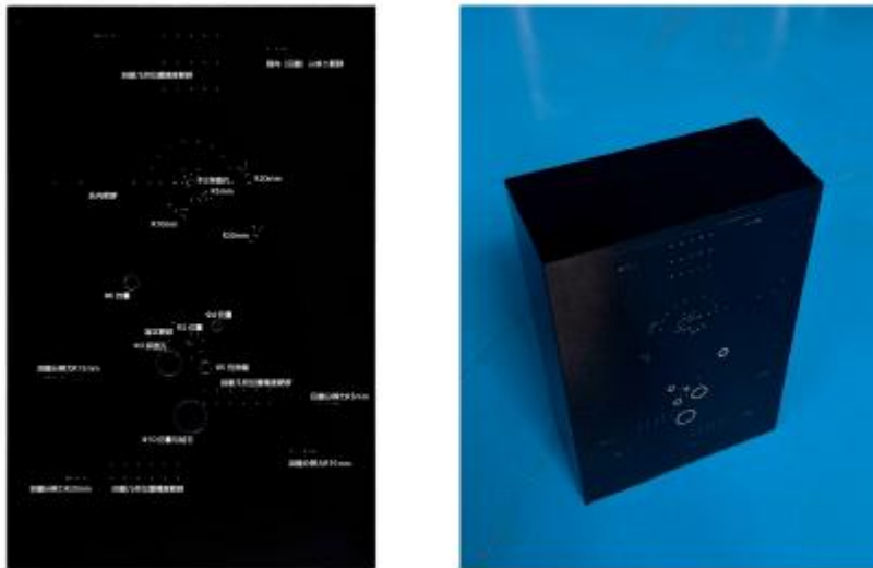
Figure A.5 Real Photo of KS107QN-4A Endocavity Ultrasound Scanning Phantom
