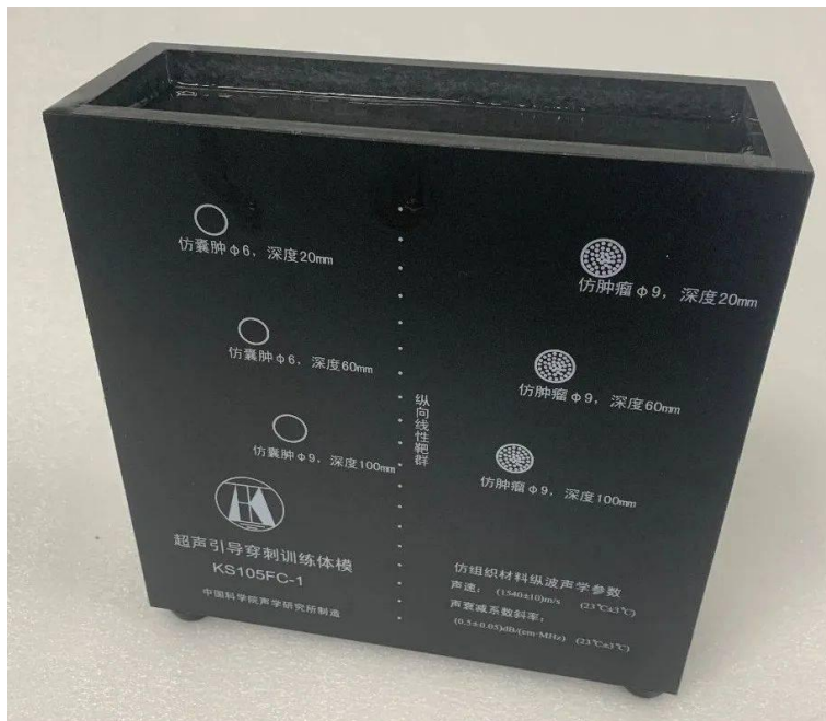
Figure 1. Photo of the appearance of the KS105FC-1 type ultrasound-guided puncture training model
