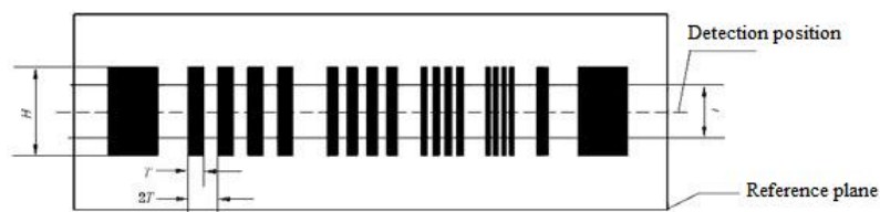
Explanation: T - Thickness of the thin slice: Also the width of the gap between adjacent thin slices; H - Height of the thin slice; t - Slice thickness for CT scanning.
